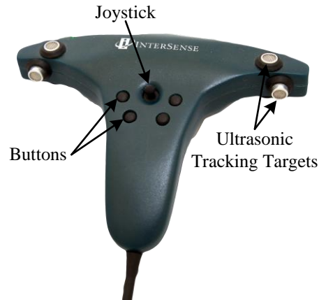
Figure 2.8: One type of wand (the Intersense IS-900) used to interact with virtual reality.
